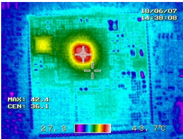
Figure 5: G2 528 MHz Full Load IR view
